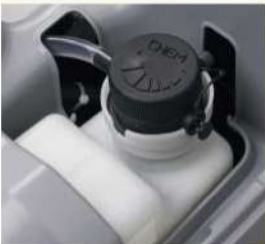
DETERGENT TANK WITH FLOW ADJUSTMENT TAP
